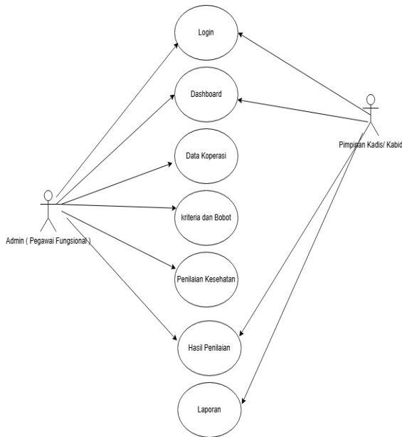
Gambar 2. Use Case Diagram Sistem
